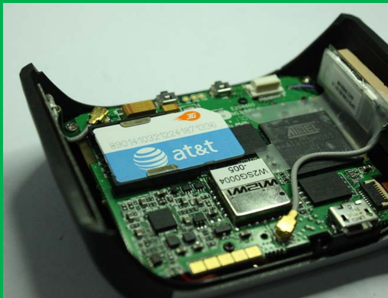
Fig8. Fully insert SIM card into the card holder
