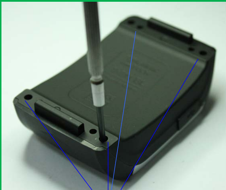
Fig6. Unscrew 4 rear case screws
