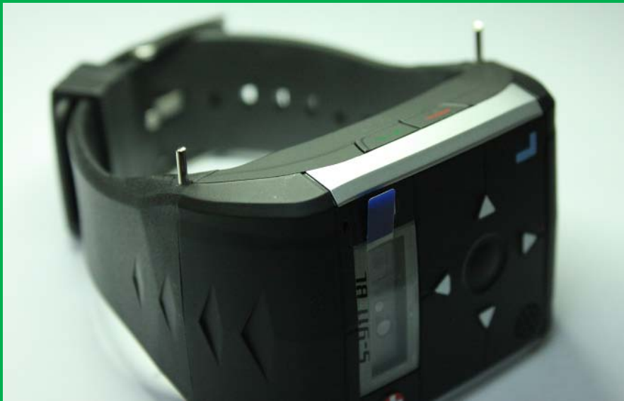
Fig4. Example of 2 pins sticking out of the wristband
